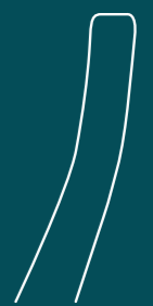
CROSS SECTION OF RIMLESS TOILET
