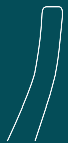
CROSS SECTION OF RIMLESS TOILET
